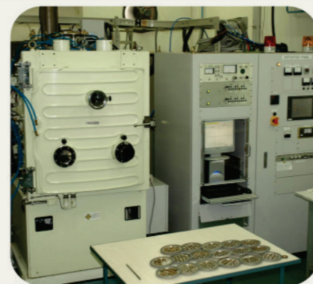
Multilayer Vacuum Coating Plant
